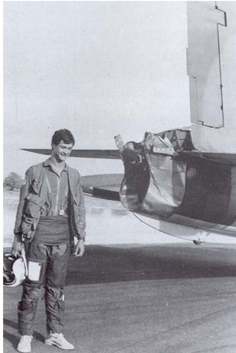
Damaged Impala Mk II jet pipe as a result of direct SA -7/14 hit
