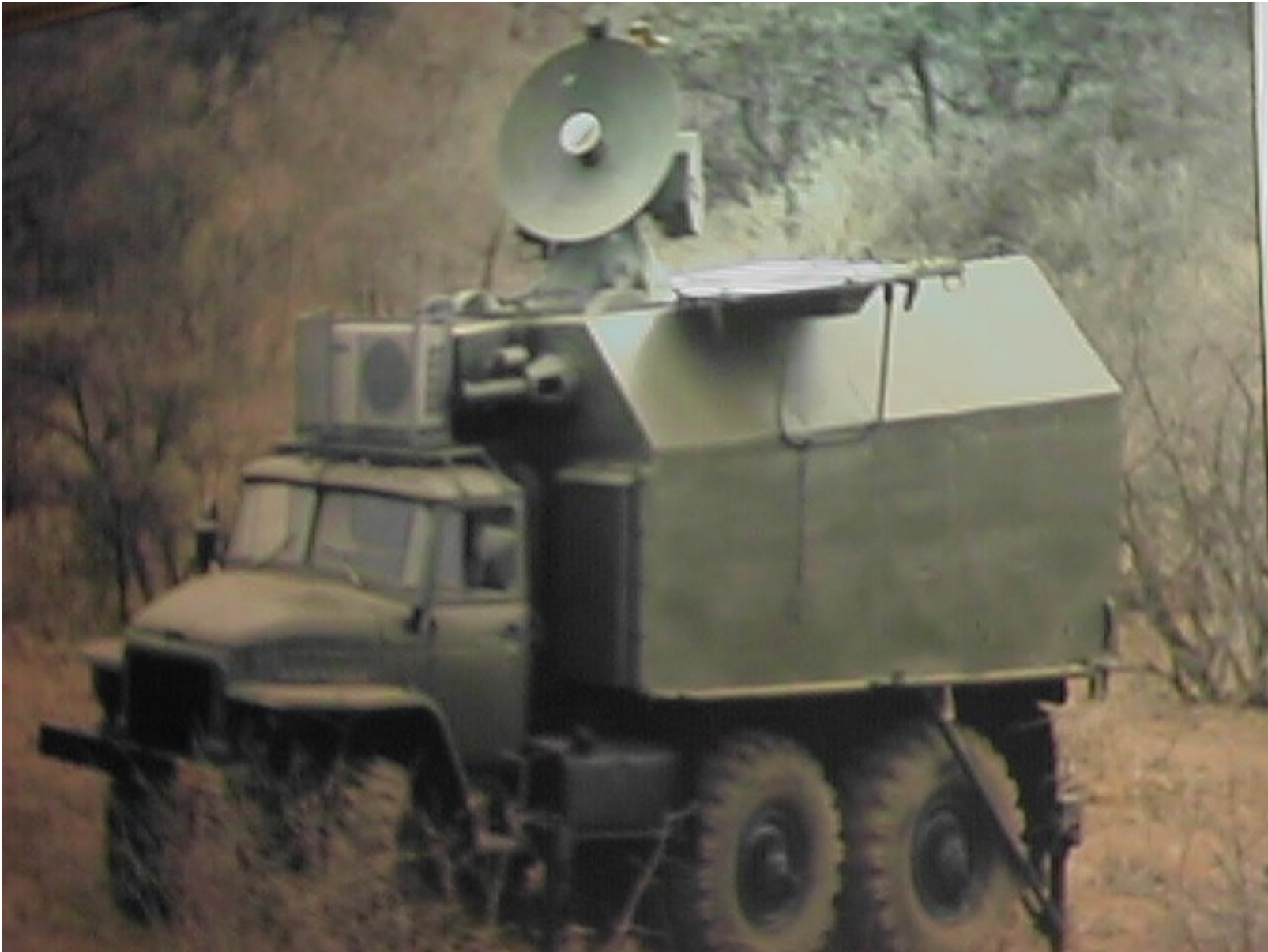
57mm AAA Fire Control Radar i.e. S – 60 “Flapwheel”
