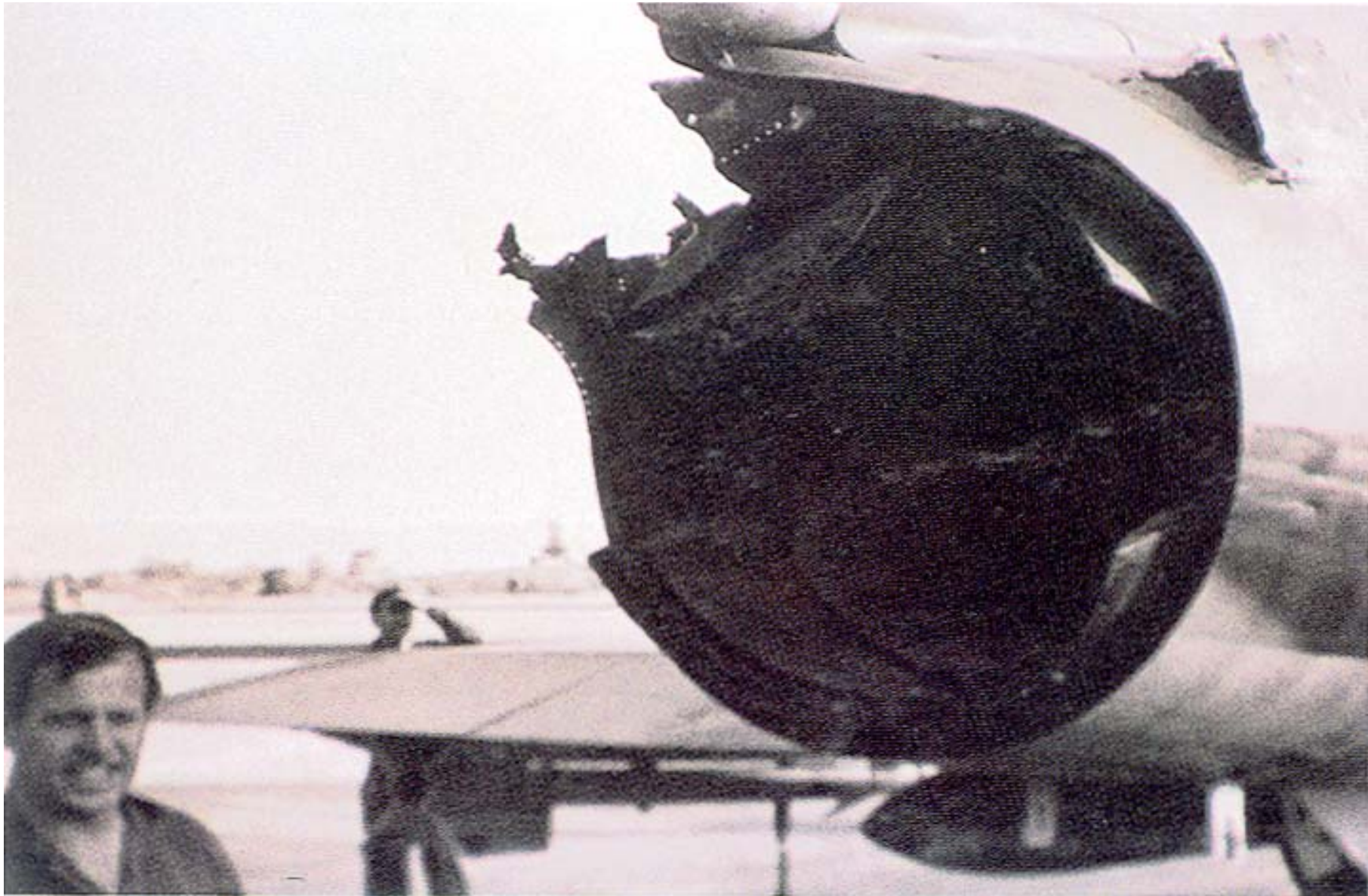
Damaged Mirage III CZ tail as a result of a direct SA – 7 hit
